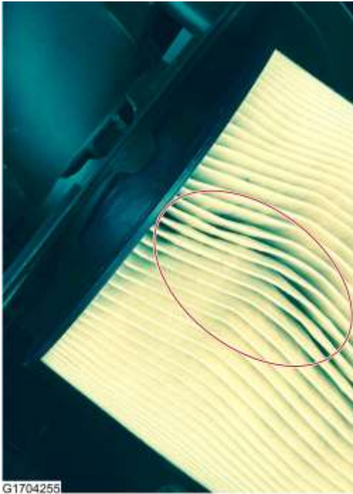
Air cleaner element misfitted
